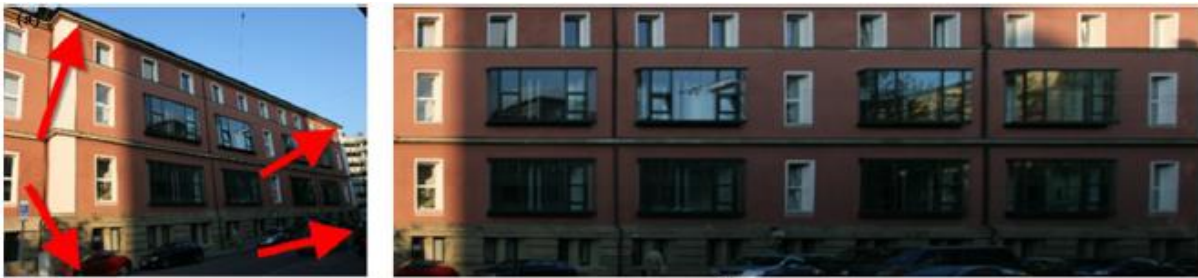
Figure 1. Four points must be selected on the photo (a) and each point provides 2 independent equations.
