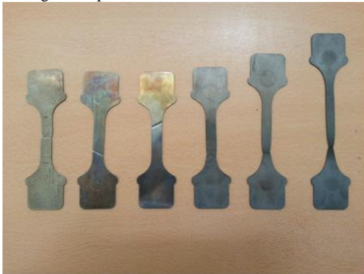
Fig. 5. Failure modes of tensile specimens at elevated temperatures (20 to 800 °C)
