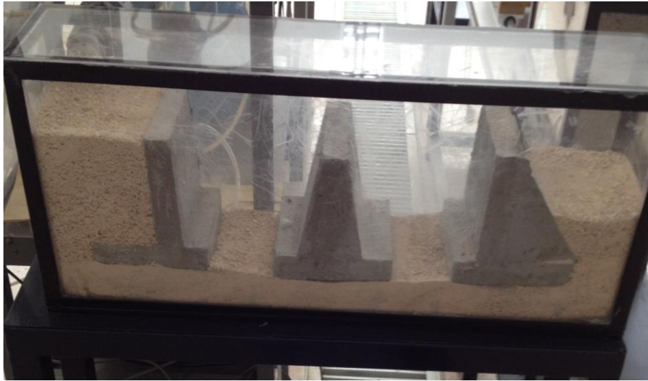
Figure 1. Retaining wall model
