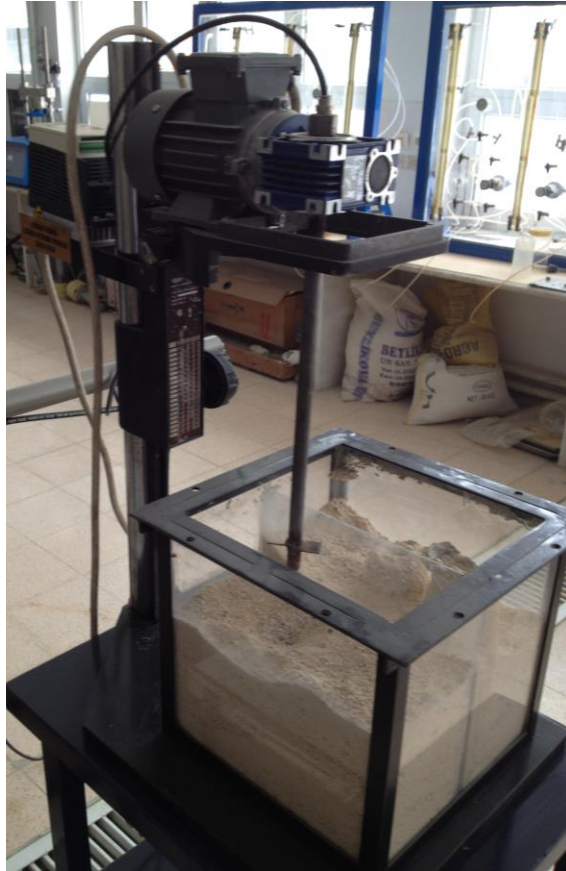
Figure 3. Deep soil mixing machine model
