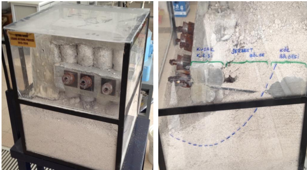
Figure 2. Deep excavation support system with anchorage model
