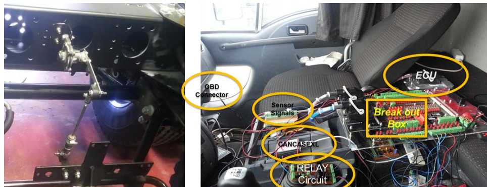
Figure 11. Sensor assembly and Electronic Circuit Layout in Cab
