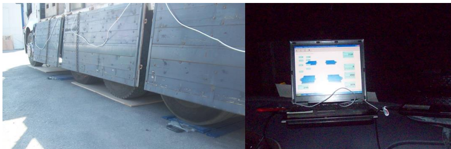
Figure 7. Training Data Collection Tests (Axle Loads and Sensor output)
