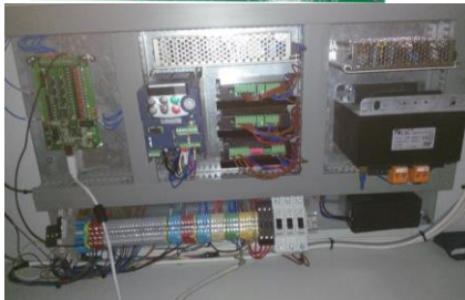
Figure 9. 3 axes USB controller board panel
