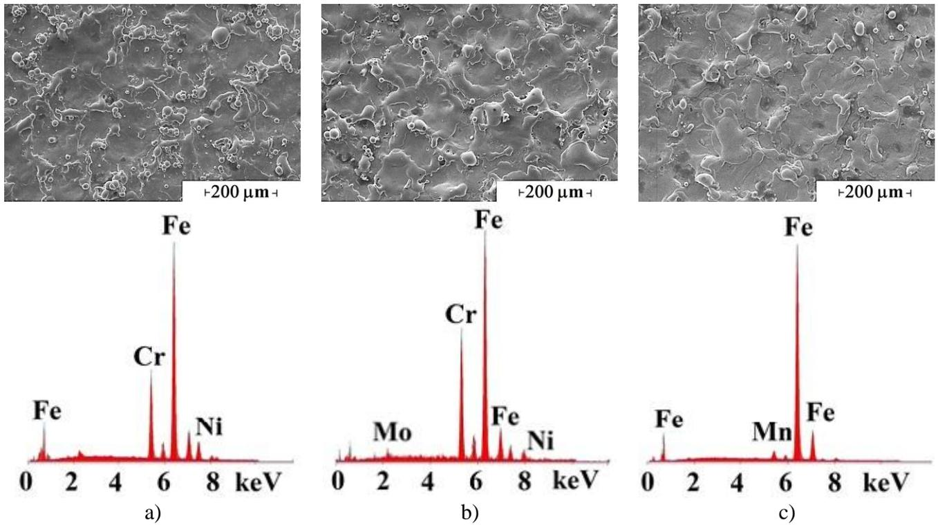
**Figure 1.** EDM'ed surfaces. Pulse-on time=12μs, Tool electrode: Copper.
