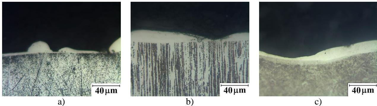
**Figure 7.** Optical section views of analyzed samples. Pulse-on time=100 $\mu$ s, Tool electrode: Copper .
