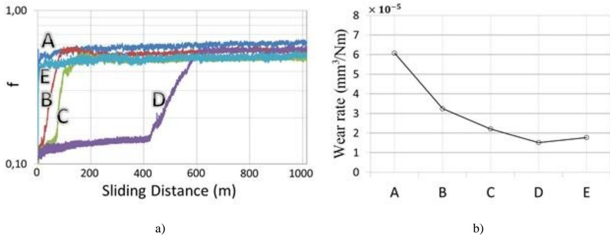
**Figure 5.** Wear rates and friction coefficients for polished and EDM'ed 1.2738 samples
