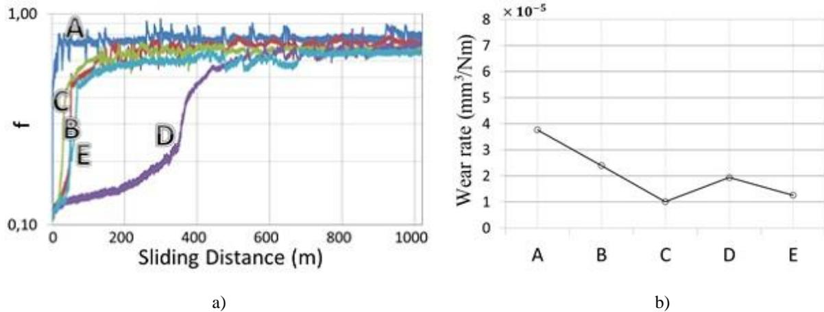
**Figure 4.** Wear rates and friction coefficients for polished and EDM'ed 1.4442 samples
