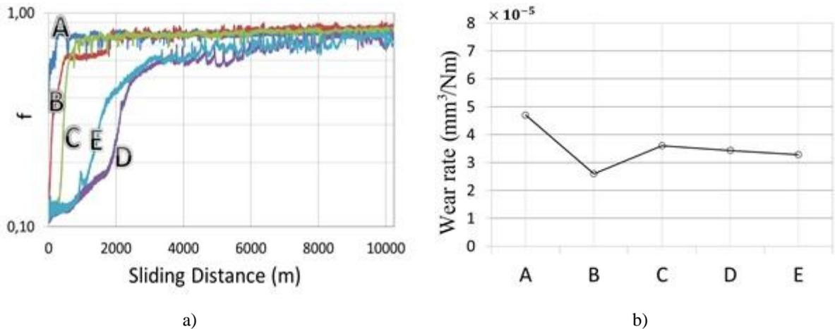
**Figure 3.** Wear rates and friction coefficients for polished and EDM'd 316L samples.
