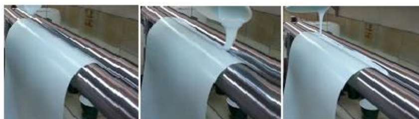
Figure 3. The preparation of coated fabric with PU/MOF-199 nanocomposite
