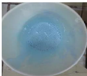
Figure 2. The photograph of PU/MOF-199 nanocomposite solution containing 5 wt.% of MOF-199
