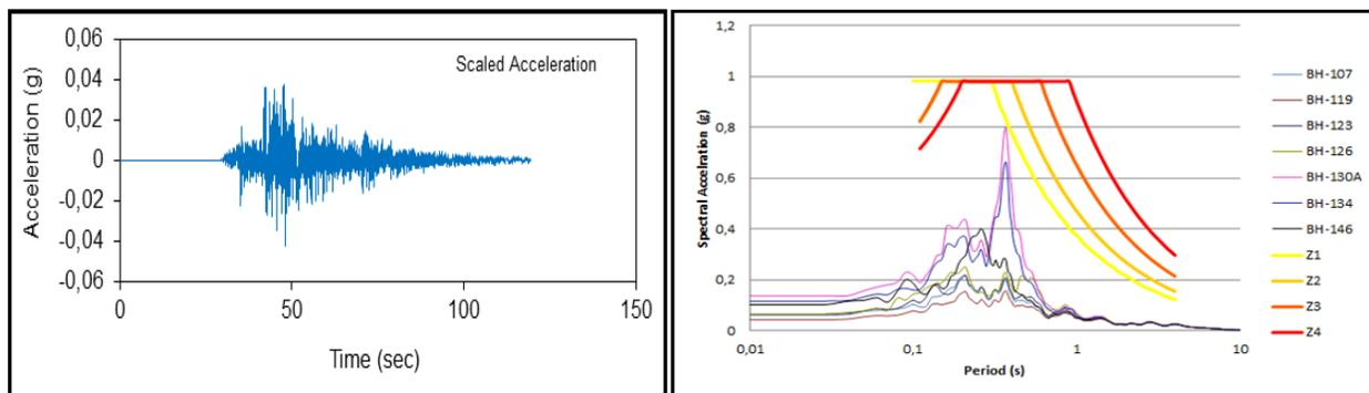
**Figure 3.** a) Record of accelerograph of horizontal component of The earthquake Kocaeli 1999 at IBPWS station obtained from PMDEMPIS online virtual data center, b) Exemplary surface spectral acceleration–period relationships belonging to various boreholes of the investigation area and comparison of the earthquake Kocaeli 1999 elastic behavior acceleration spectrums with Turkish Earthquake Regulation Spectrums (2007 elastic medium).
