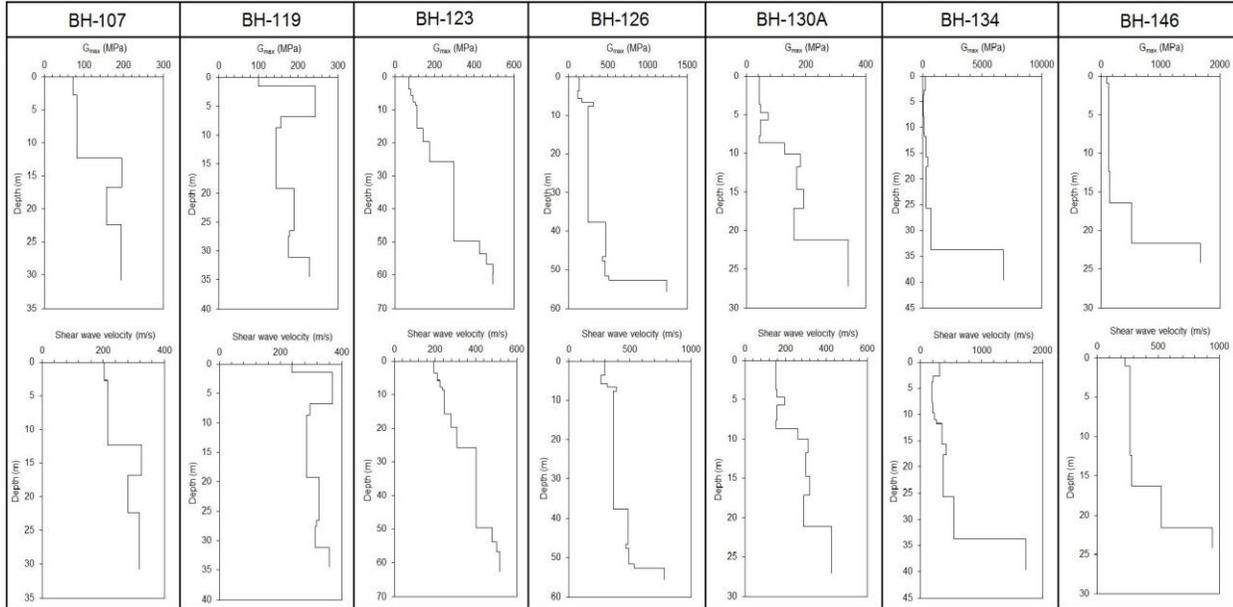
Figure 5.  $G_{max}$ - depth and shear stress - depth variation graphics of the boreholes (from EERA)
