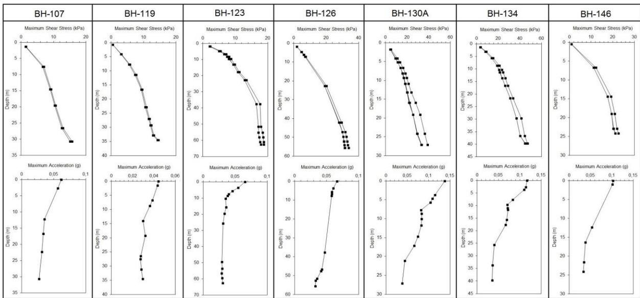
**Figure 4.** Max shear stress variation with depth of the boreholes (Results of the 1D ground response analysis performed with EERA)
