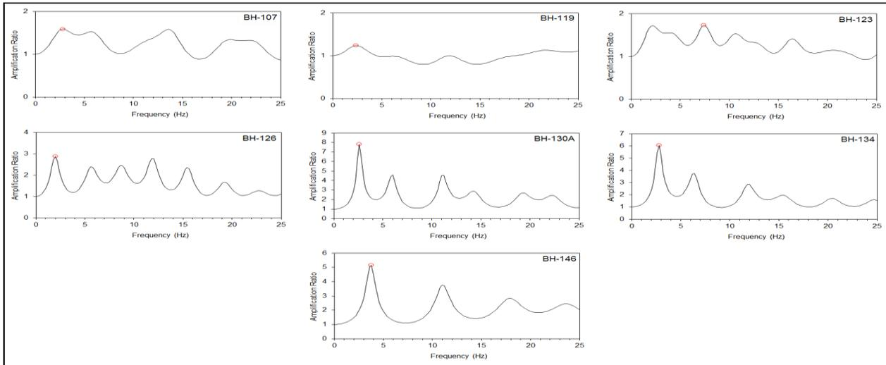
Figure 6. Amplitude ratio values of acceleration in boreholes.
