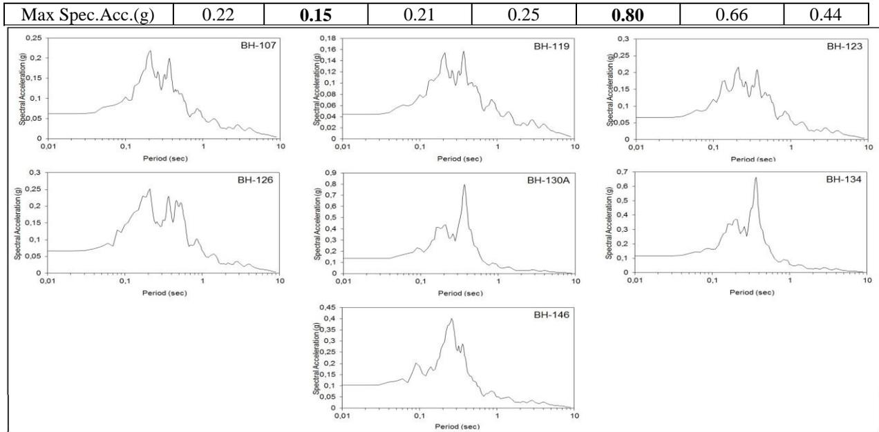
**Figure 7.** Spectral acceleration and Period relationship of the boreholes (from EERA)
