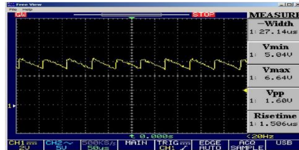
Figure 4. Rectified and pulsed high voltage supply to the reactor. The real value of peak voltage is 50760 V by setting the selector switch to the level 6. But the induced voltage can be seen as 1.6 V pp .
