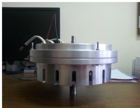
Figure 3. Mounted axial flux permanent magnet brushless dc motor prototype
