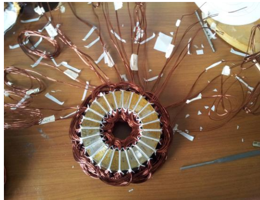
Figure 2. Distributed winding on stator steel core
