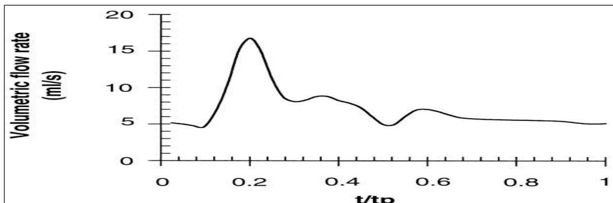
Figure 1. Volumetric flow rate-dimensionless time curve of blood flow through human carotid artery
