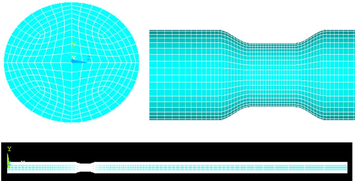
**Figure 3.** Web structures of constricted carotid artery at the inlet section and at the constricted region and artery's image along its length
