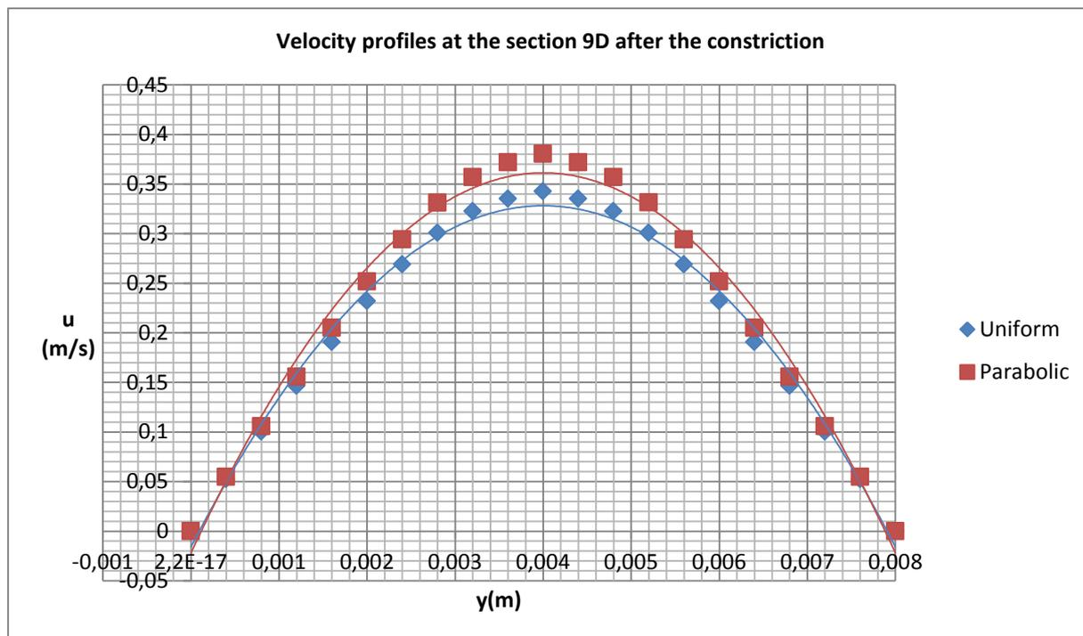
**Figure 7.** Velocity profiles at the section 9D distance after the constriction
