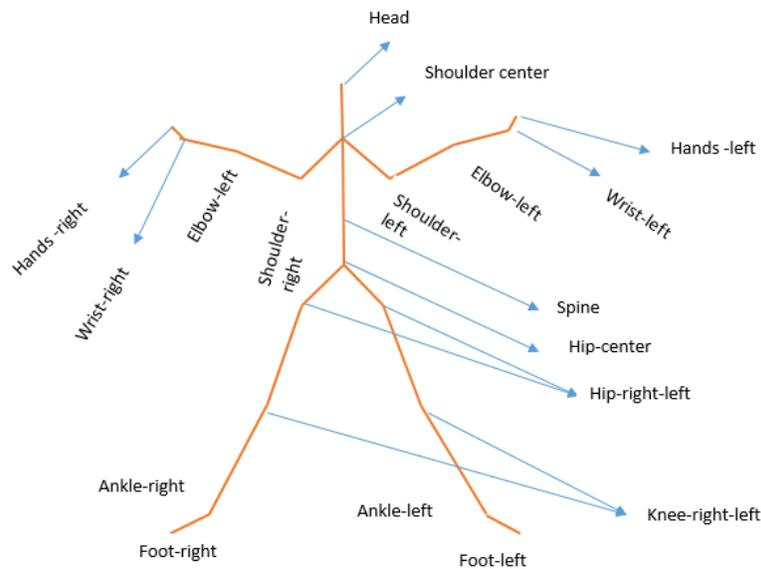
**Figure 3.** Human skeletal joints that Kinect Sensor found [8]
