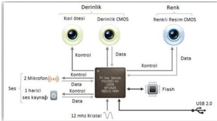
**Figure 2.** Hardware structure of Kinect sensor [8]
