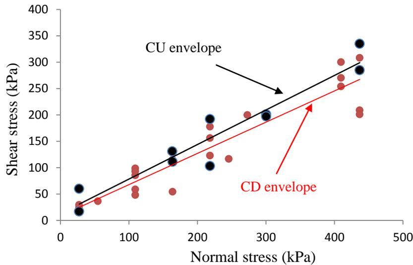
Figure 2. Failure envelopes obtained for drained and undrained shear tests.
