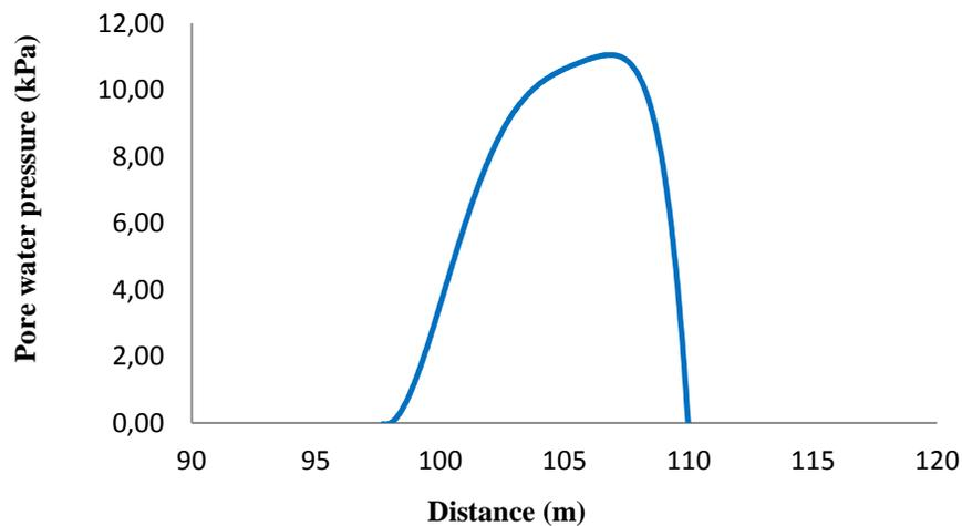
Figure 4. Pore pressure distribution assigned across the failure surface needed to reach limit equilibrium to start a consolidated-drained failure for a 20 m slope.
