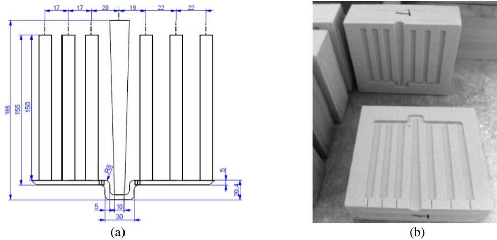
**Figure 1.** a) The dimension of the mould b) The sand mould used in the casting trials
