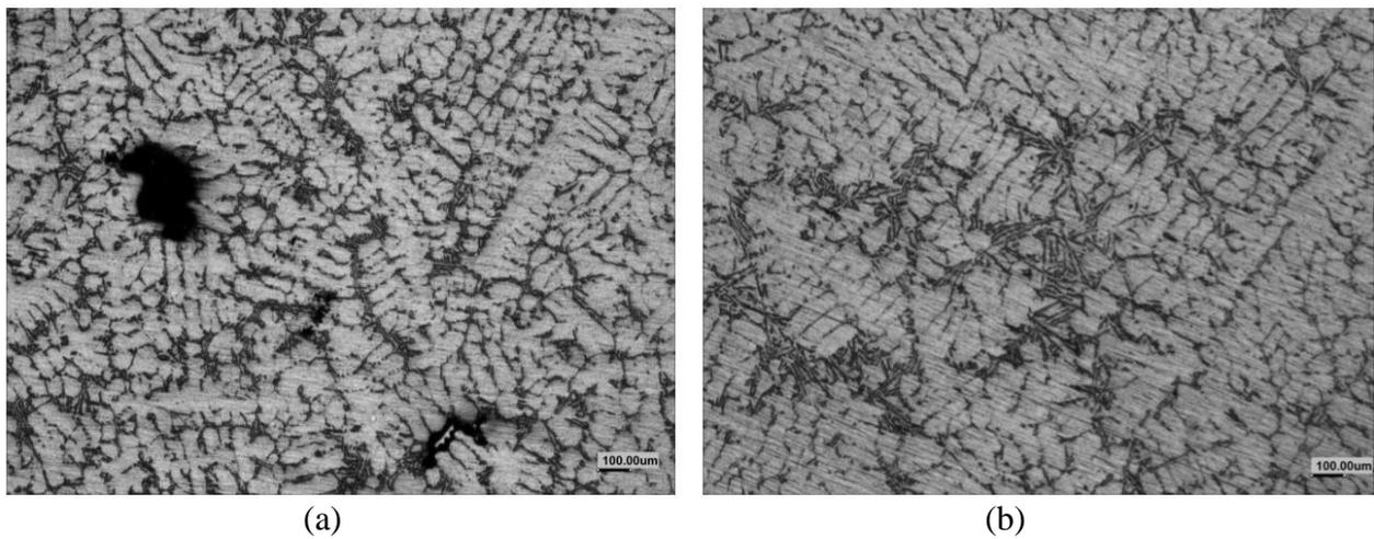
**Figure 4.** Microstructures of the as-received alloy
