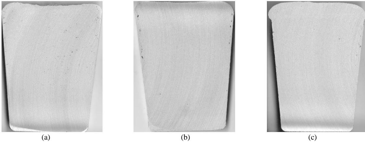
**Figure 3.** RPT samples produced from the degassed melt (a) as-received, (b) Sr modified, (c)  $\text{AlB}_3$  grain refined
