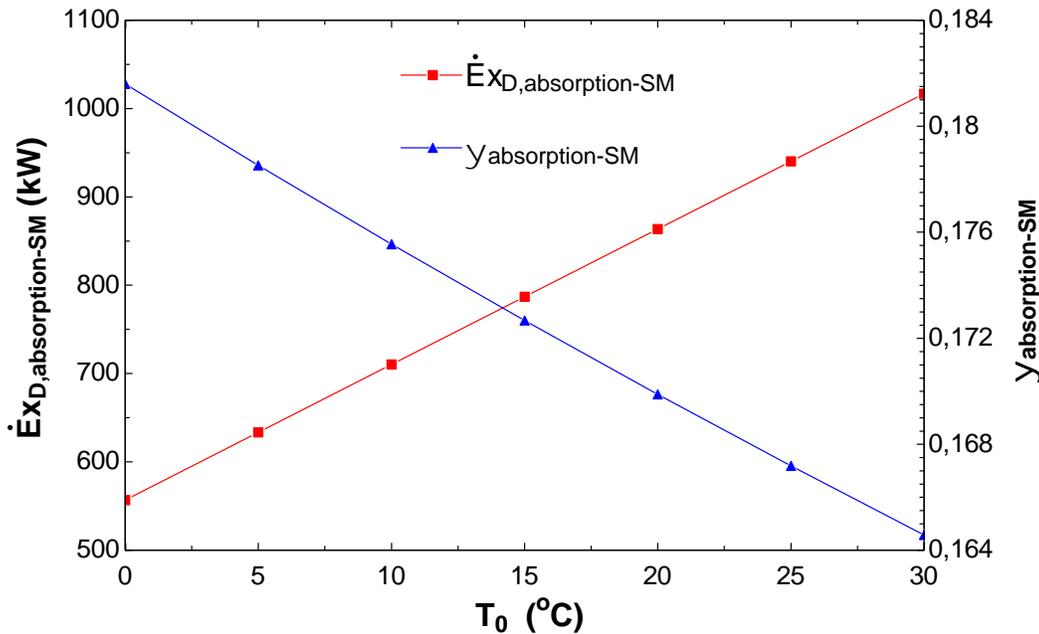
**Figure 2.** Exergy destruction rates and exergy efficiencies of the double effect absorption system depending on the reference temperature changes
