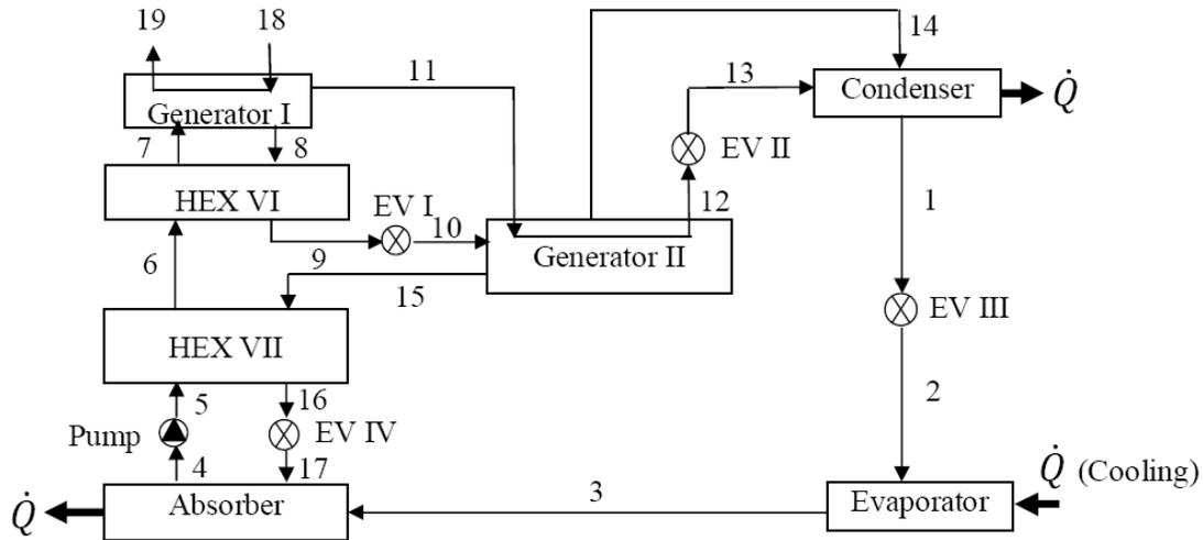
**Figure 1.** A schematic diagram of a double effect absorption cooling system
