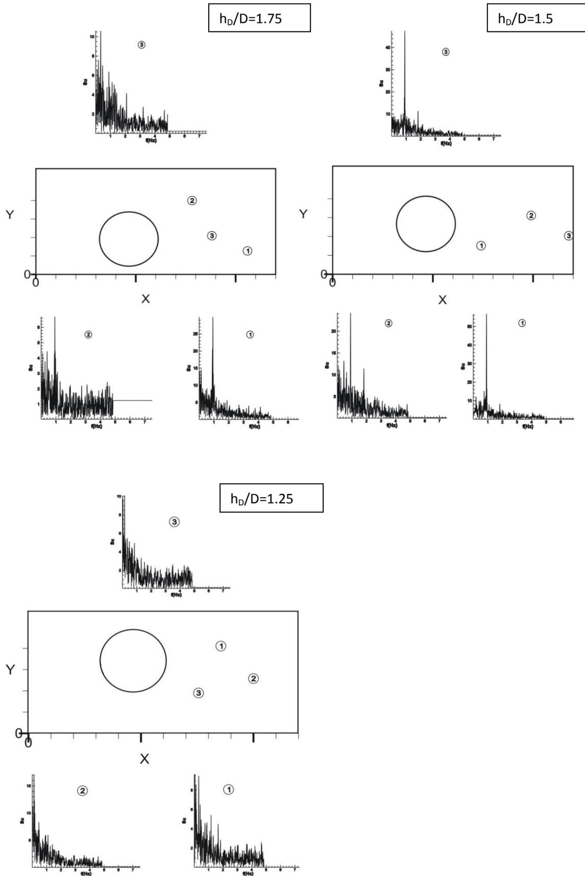
**Figure 4.** Spectra of streamwise velocity fluctuations evaluated at various locations in the flow field for  $h_D/D=1.25$  and 1.5, 1.75
