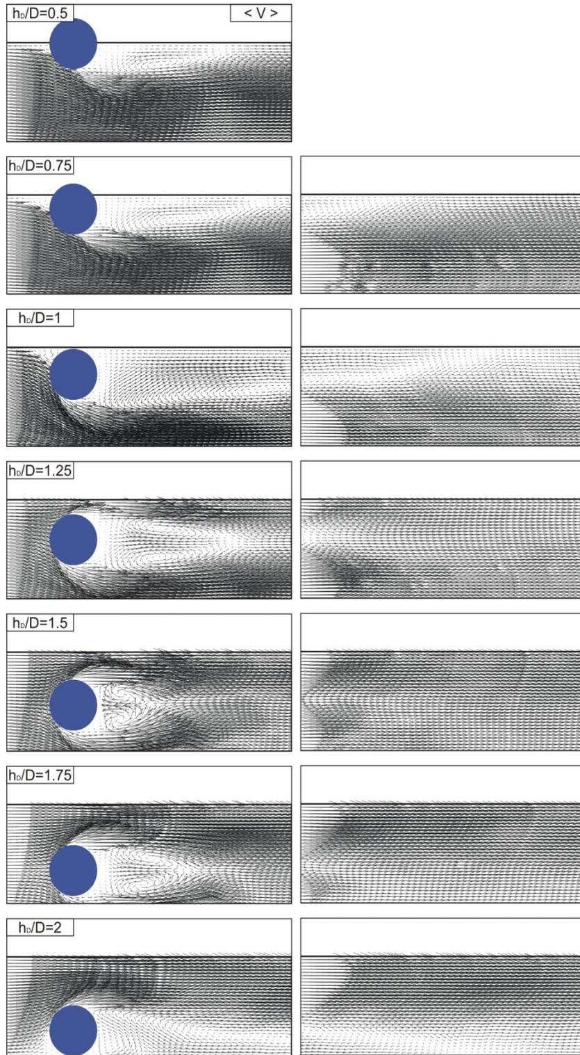
**Figure 2.** Velocity vector field for horizontal circular cylinder
