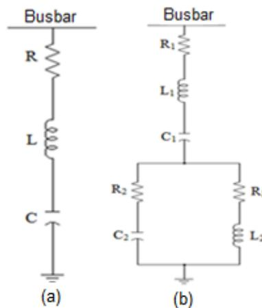
**Figure 1.** Passive filters a) Single tuned, b) Doubled tuned
