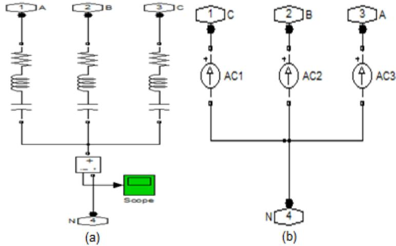
**Figure 6.** (a) 3th harmonic filter connection diagram, (b) 5th harmonic producing current sources
