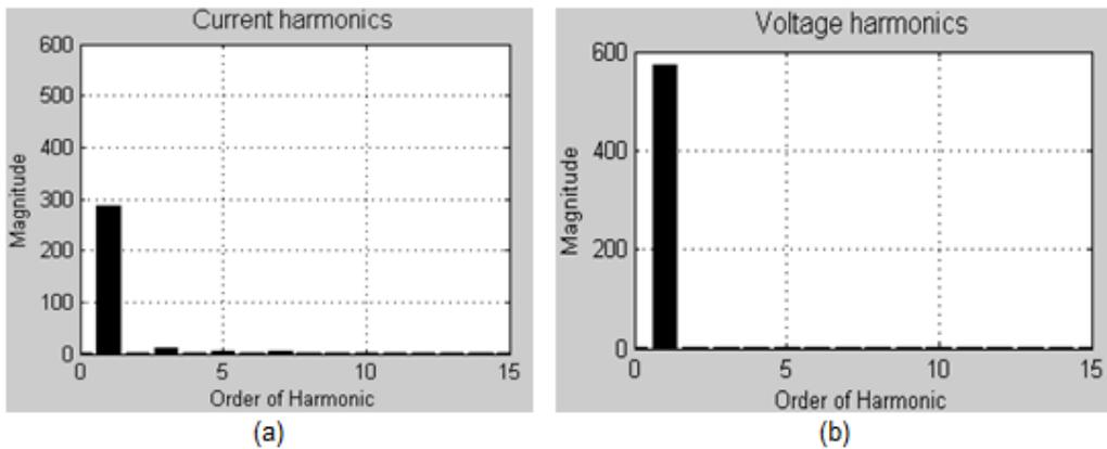
**Figure 8.** (a) Current harmonics of filtered system, (b) Voltage harmonics of filtered system
