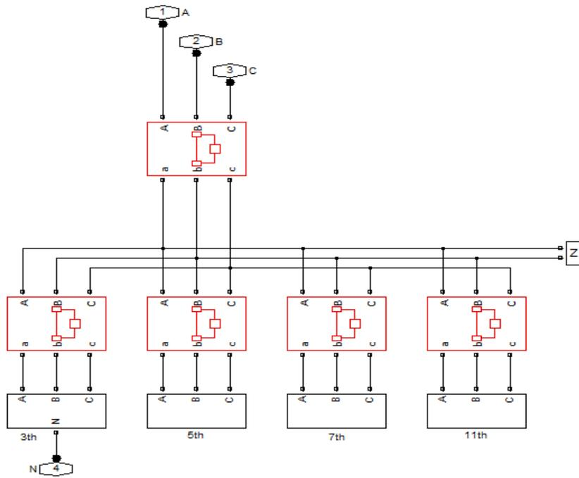
**Figure 5.** Filter connection diagram
