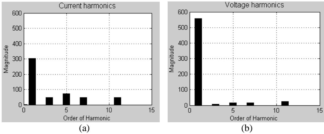
Figure 4. (a) Current harmonics of unfiltered system, (b) Voltage harmonics of unfiltered system
