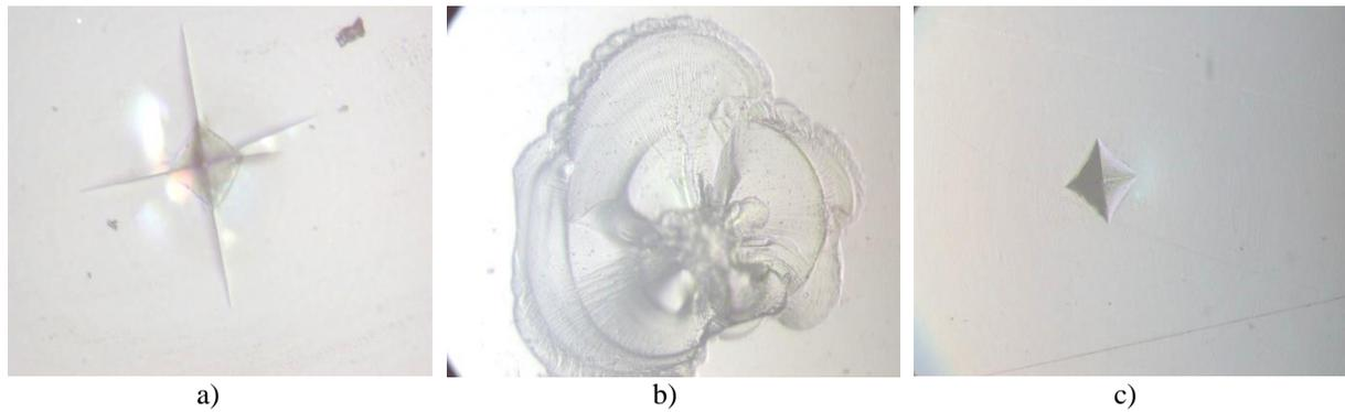
**Figure 3:** Micrographs showing three glasses indented by the same load 9.8 N
