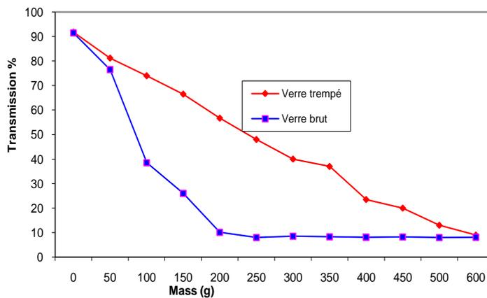
**Figure 2:** Comparison of transmission loss of two glasses treated by annealing and thermally tempered
