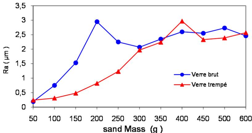
**Figure 1:** Variation of the roughness  $R_a$  (microns) of annealed glass and thermally toughened glass versus the projected mass of sand
