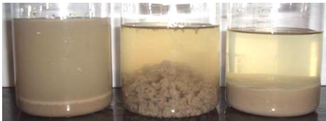
a) No chemical b) Long polymer c) Short polymer Picture 2: Effects of coagulants/flocculant on a recycled pulp slurry.
